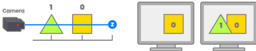
(Fig. 3.1.5a. As we can see from the picture, the triangle is drawn on the screen first due to it being farthest from the camera. In the end, the square is drawn, and together generate 2 draw calls)
