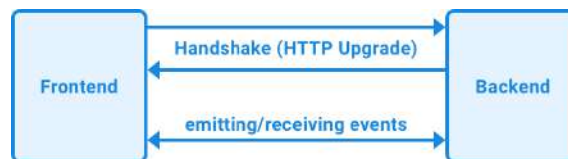
Figure 13.2 – Establishing a connection with Socket.IO
