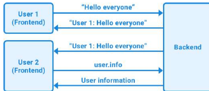
Figure 13.3 – Emitting and receiving events with Socket.IO
