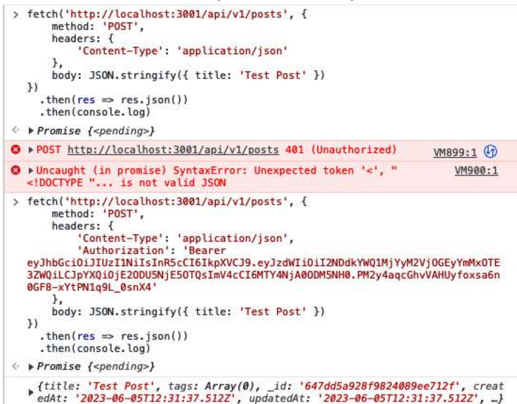
Figure 6.4 – Attempting to access a protected route without a JWT and then with a JWT
