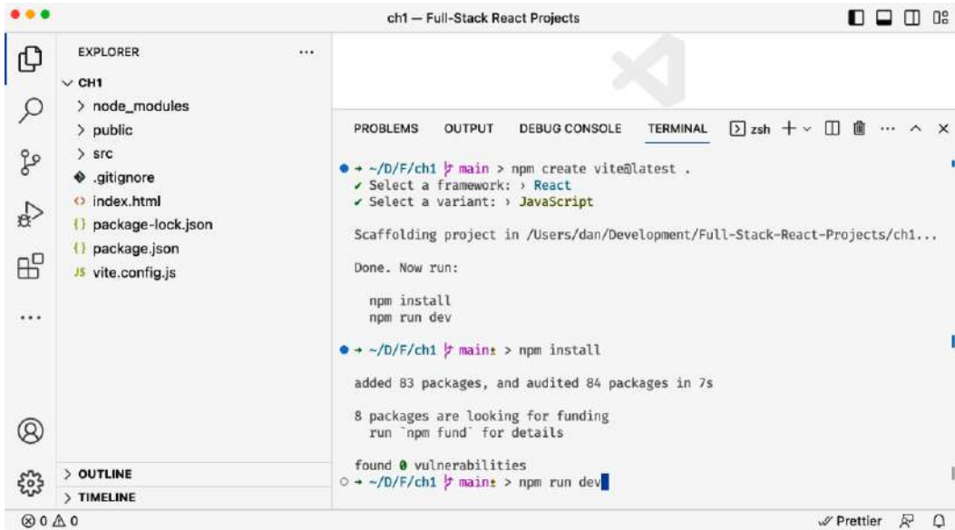
Figure 1.4 – The Terminal after setting up a project with Vite and before starting the dev server
