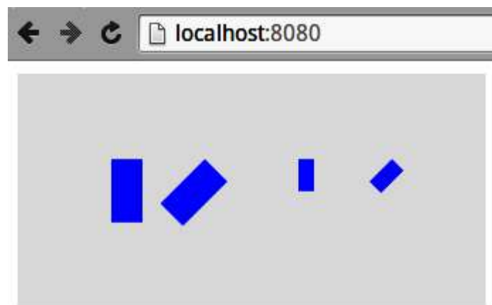
Figure 4-18. Some SVG transforms: rotate(45) , scale(0.5) , scale(0.5) , then rotate(45)
